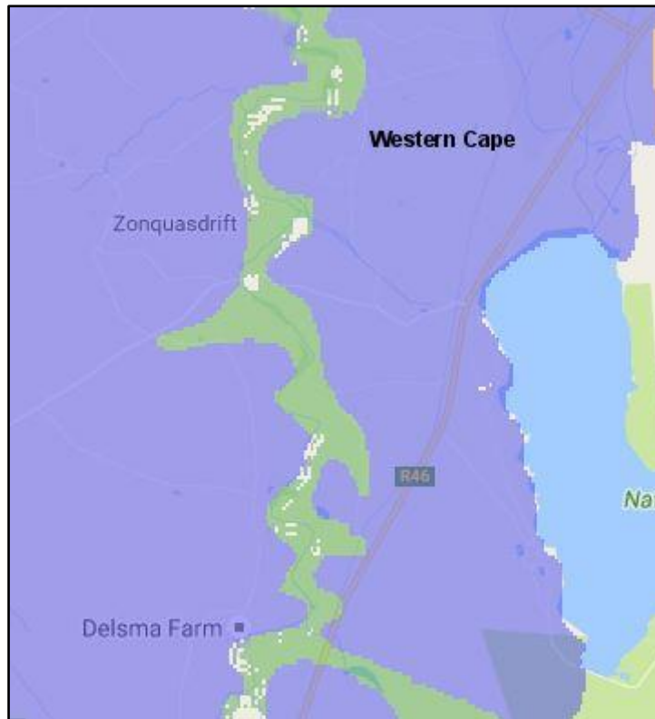
Figure 4: The SAHRIS Palaeo sensitivity map indicates that the pipeline route will run through the blue area on the map which is considered to have low sensitivity. The green area along the Berg River is considered to have moderate sensitivity and a desktop study is required for developments along the river.
