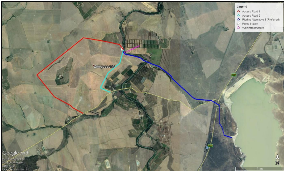
Figure 2: The various infrastructural components of the project are illustrated in this map. There are two road options (red and turquoise) and the blue line indicates the preferred pipeline alternative to the Voëlvele Dam.
