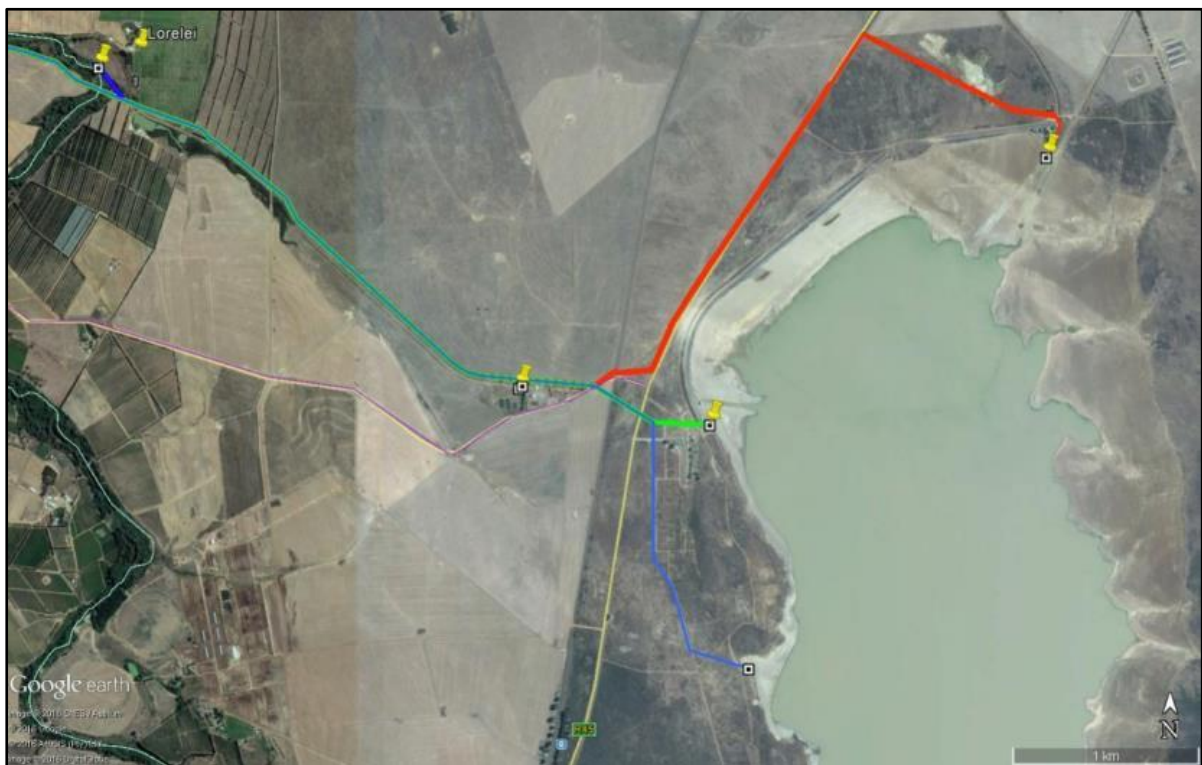
Figure 3: Indicates the various alternative pipeline discharge options (Option 1 = red, Option 2 = green, Option 3 = blue is the preferred option) into the Voëlvele Dam.
